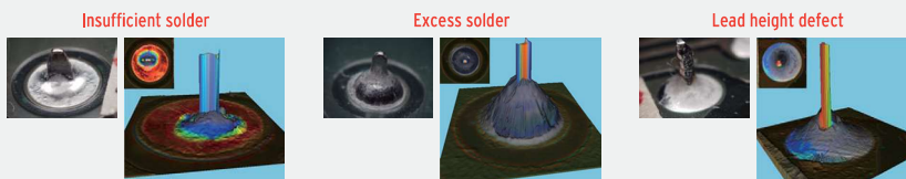
Flow solder/insertion component inspection examples
