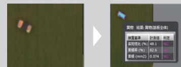
Foreign object (0402 scattered chip) detection example
